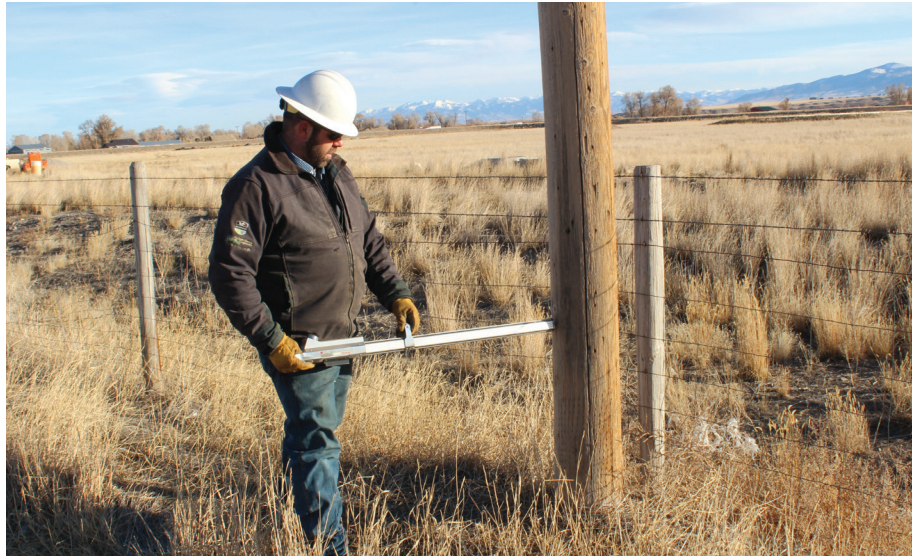
Pictured is lineman Cody Tater demonstrating a pole-testing drill. | VIGILANTE FILE PHOTO
